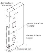
Note 1: Align the template along the vertical center line of the mortise (F) at the desired handle height, and tape it to door.
