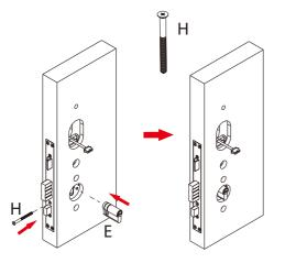
Note: Install lock cylinder in right direction, then tighten screw (H) to fix it.
