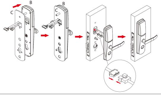
6. Install mounting plate (K) with gasket (C) on the door
