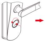
Press the cover on key hole and contrarotate it at 30° to remove the cover.
