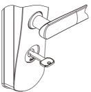
Insert the key into key hole and rotate it.
